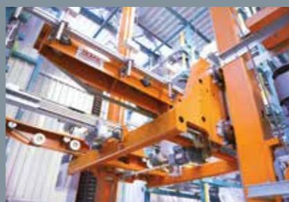
Storage and retrieval machines
